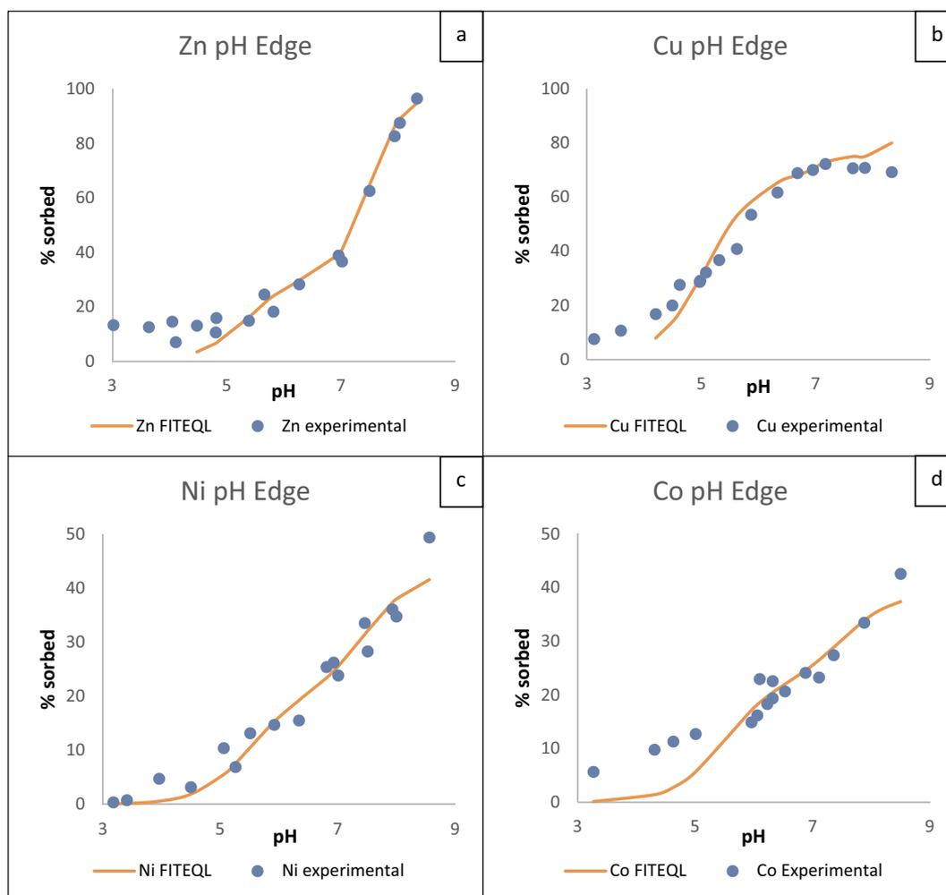
Fig. 2. (a–d): Zn pH edge in terms of % adsorption over the pH range studied, plotted alongside the FITEQL model.
