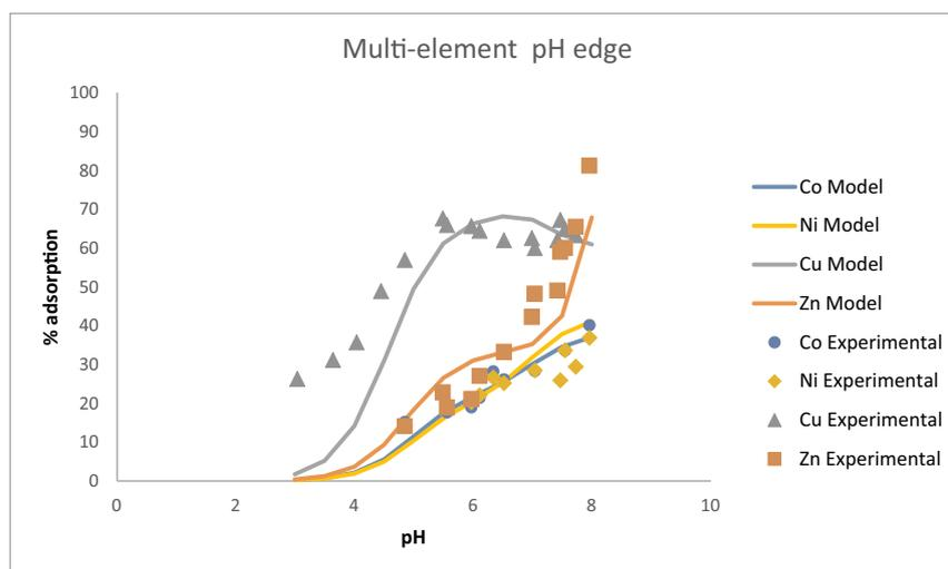
Fig. 3. Competitive adsorption of the 4 studied metals in terms of % adsorption, plotted alongside the predicted FITEQL model from the determined K values for each metal from the single element adsorption experiments.
