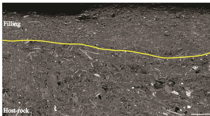
Fig. 6. Scanning electron microscopy-back-scattered electron imaging (SEM-BSE) coupled to energy-dispersive X-ray spectrometry (EDX) showing contrast in textural and mineralogical compositions within the LF comparing to the host rock. The yellow line traces the contact between the LF specimen and its host rock. It shows very clearly to the naked eye that the grain size of quartz, micas, and chlorite are coarser and more randomly distributed in the host rock than in the LF specimen. White scale bar is 1 mm.
