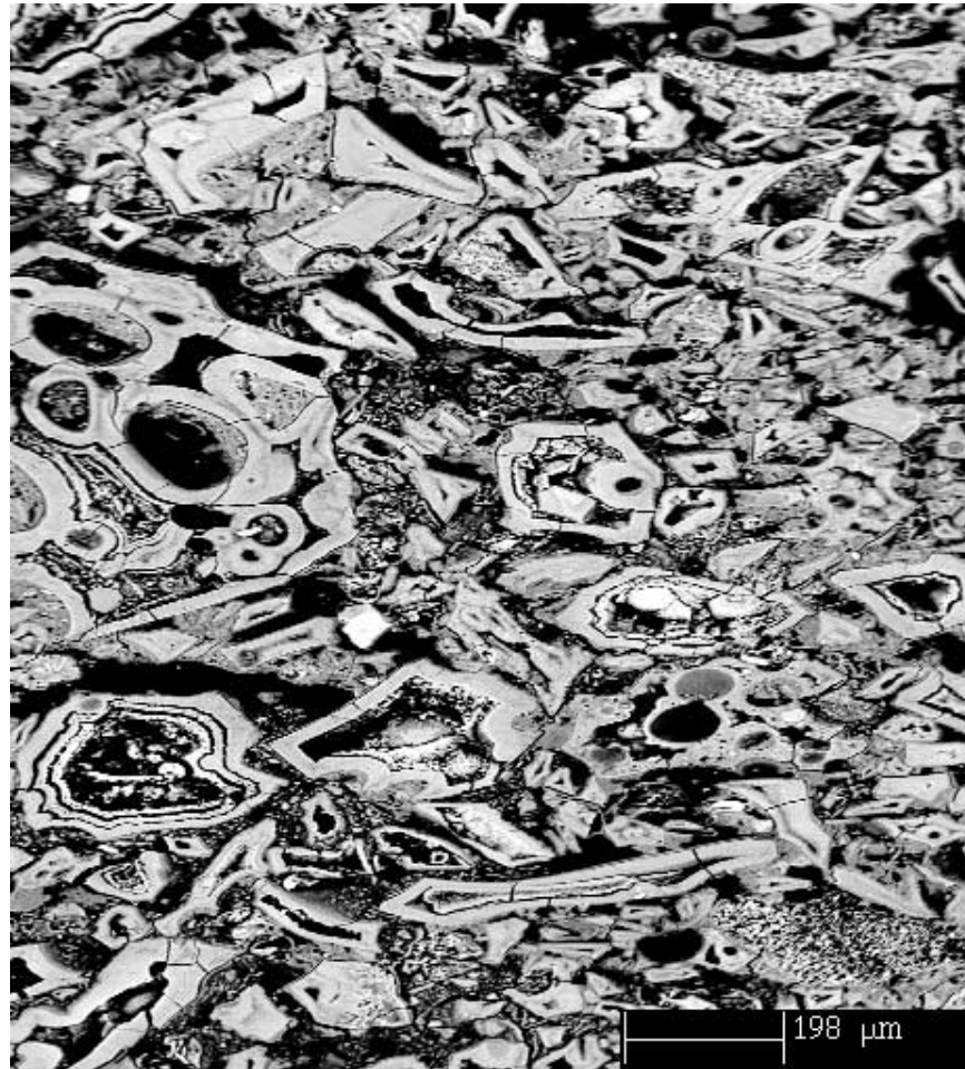
Figure 2. Backscattered electron microprobe images of highly altered tephra: (a) Low magnification image depicting relict vesicular glassy shards with banded alteration features; (b) Close-up of an individual, banded altered glass shard. The core of the shard is nearly completely dissolved. The numbers in the lower left and bottom margins of the shard refer to compositional analyses (i.e., p1–p5) presented in Table 2.
